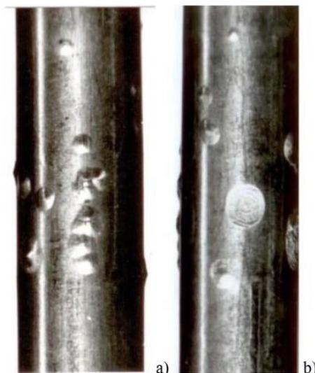
**Figure 53: Nodular corrosion (after crud removal) on CANDU fuel rod Zircaloy-4 cladding tested 90 days in TRIGA reactor using irradiation capsule. (From [283])**
