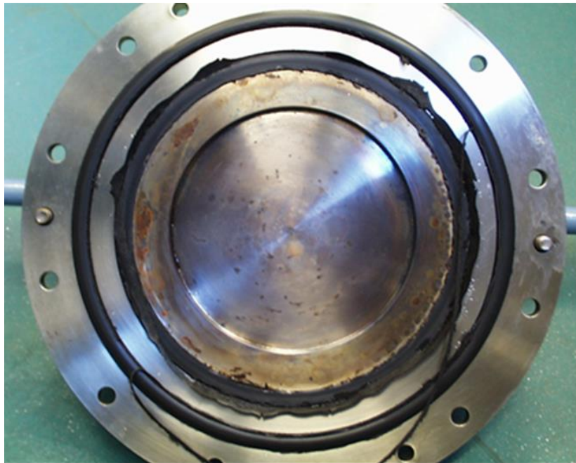
Figure 19 Aged FKM flask seal after a maximum of 204°C and a cavity pressure of 42 bar.
