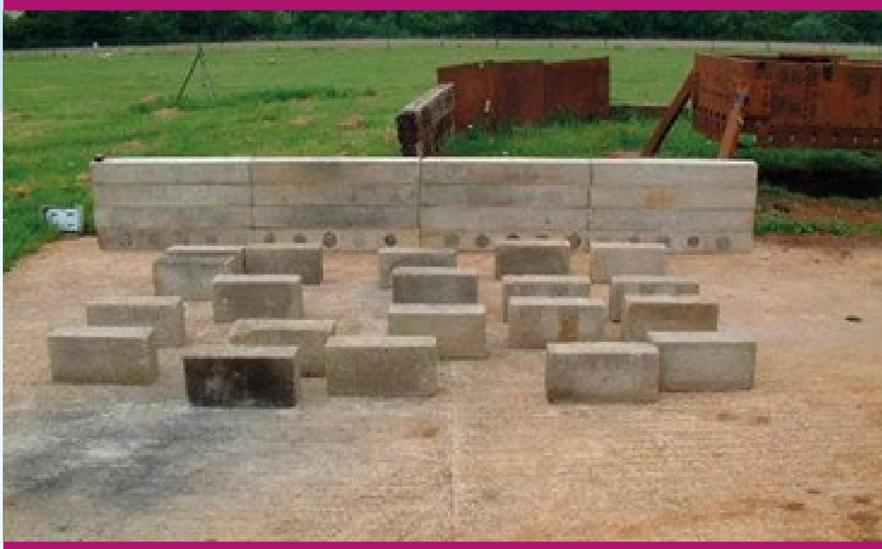
Figure 12: Scaled physical tests using scaled explosives and blast sensors
