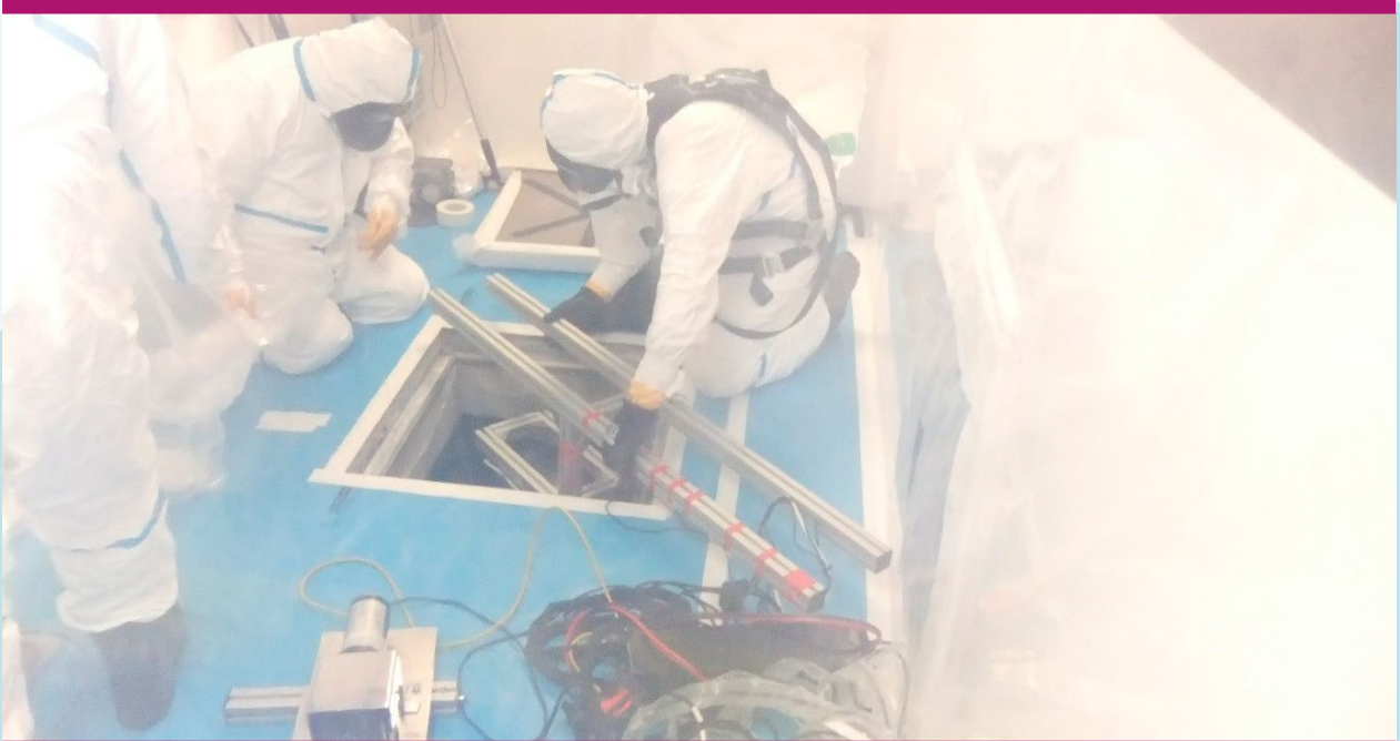
Deployment of an autonomous robot to survey a duct
