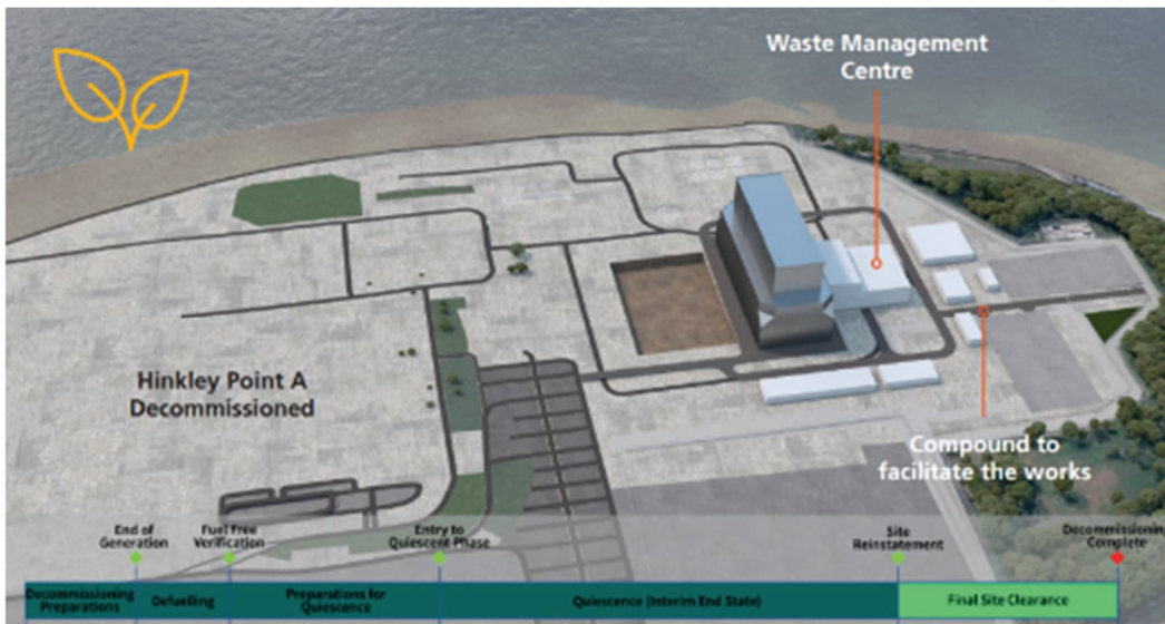
Graphic 3-9 Illustration of HPB site at the peak of Final Site Clearance activities
