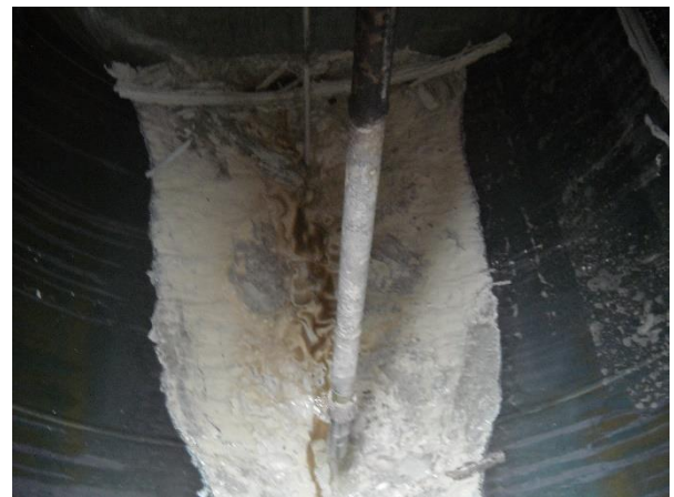
Photographs 14 and 15: The AETP Acid & Caustic Tanks draining operation, and the sludge encountered in
